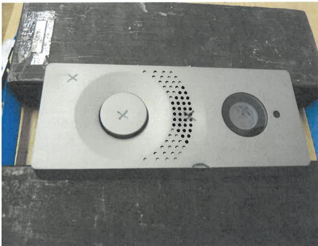
Fig. 2 Sample after the test with marked impact spots
