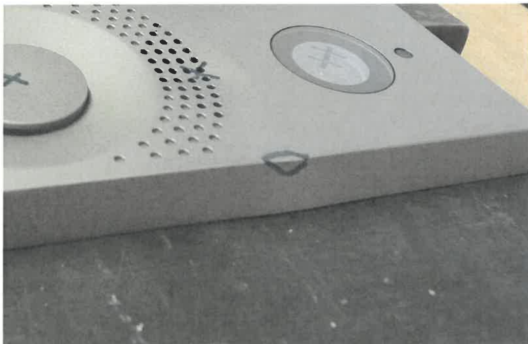
Fig. 4 Detail of the minor deformation of the cover after the impact
