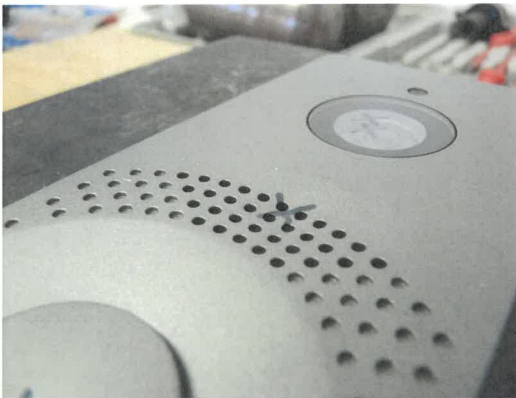
Fig. 3 Detail of the minor deformation of the cover after the impact
