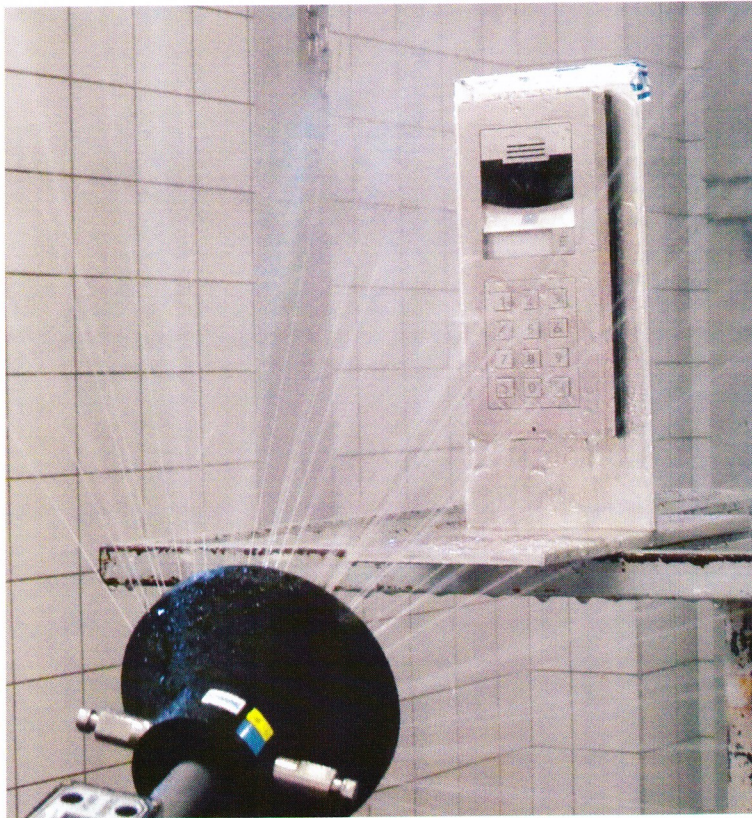
Fig. 4 - IP X4 testing (the specimen for surface installation)
